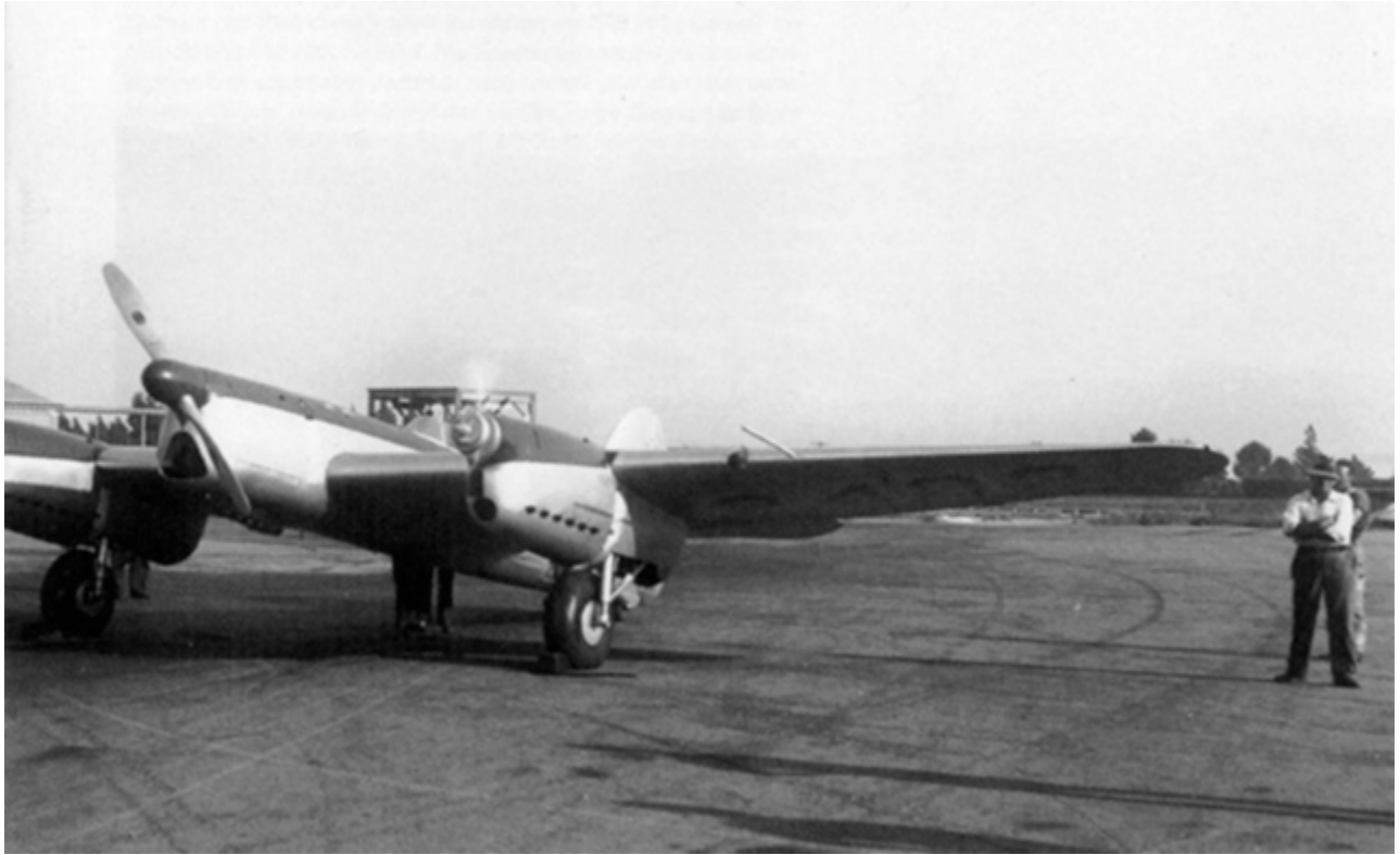
Bellanca Model 28-92 after apparently being acquired by Frank Fuller and International Aircraft Trading Co. as NX-2433. This is the color scheme it is believed to have worn when delivered to Ecuador. The props and spinners for the two outboard Menasco engines have not been installed. (Photo: Via Dave Ostrowski.)
