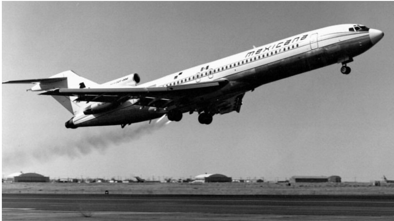
One of Mexicana's JATO-equipped Boeing 727s. (Photo: Boeing.)
