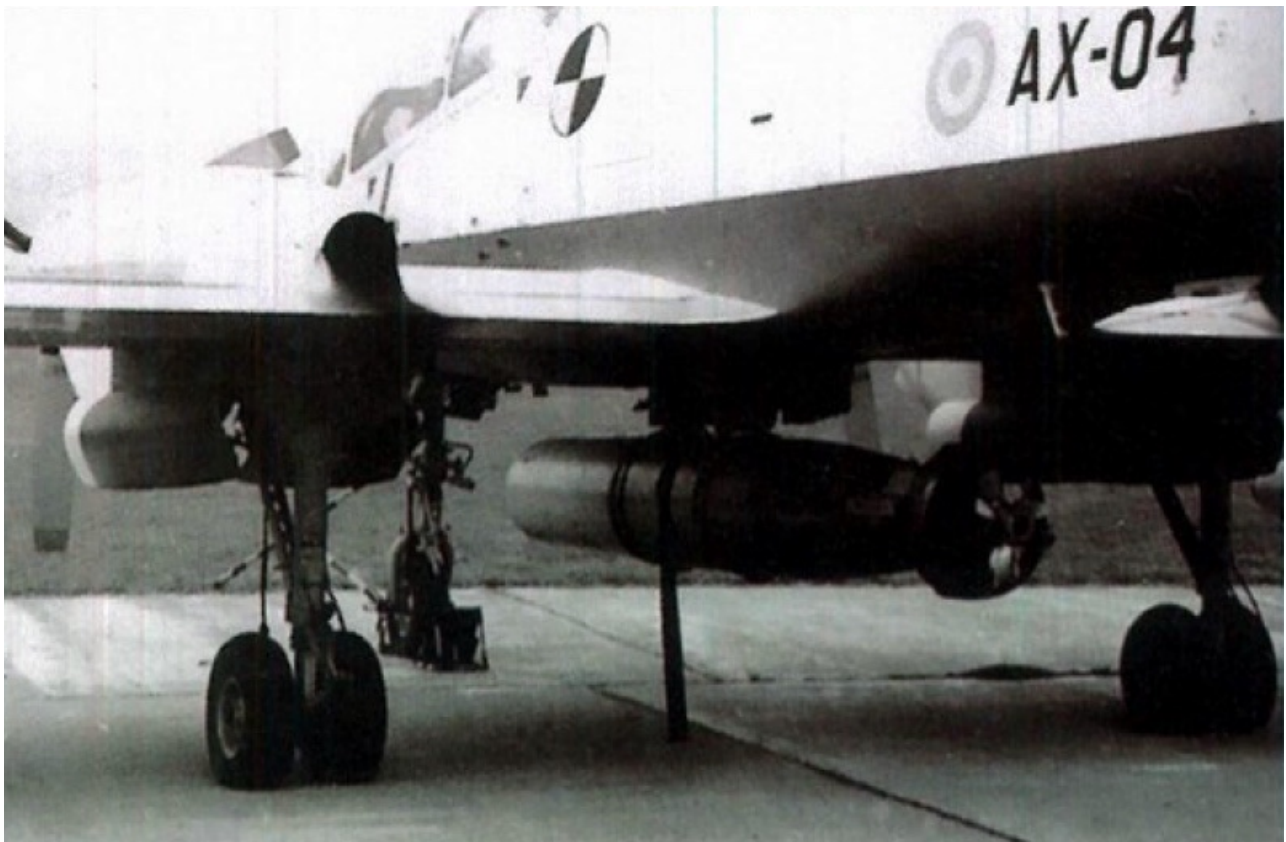
Another view of the Mk.13 torpedo, loaded on the ventral station of the IA-58A serial AX-04. (Photo: Roberto Caballero.)
