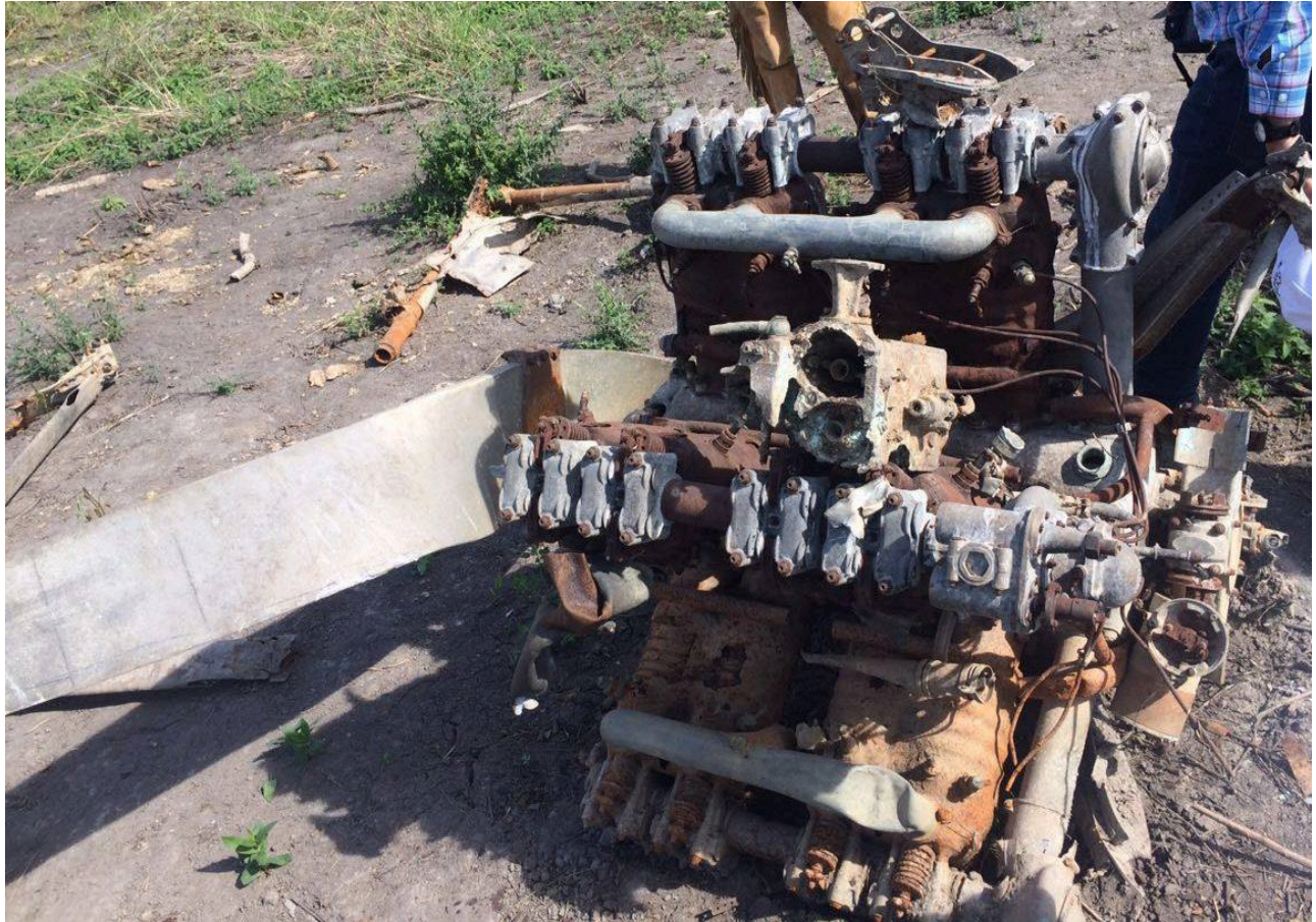
The engine of the Potez 25 T.O.E. serial 13, which was found, along with other components, in 2016 at Cañada El Carmen. Currently, these parts are being preserved at the Fortín Boquerón Museum. (Photo: Via the author.)
