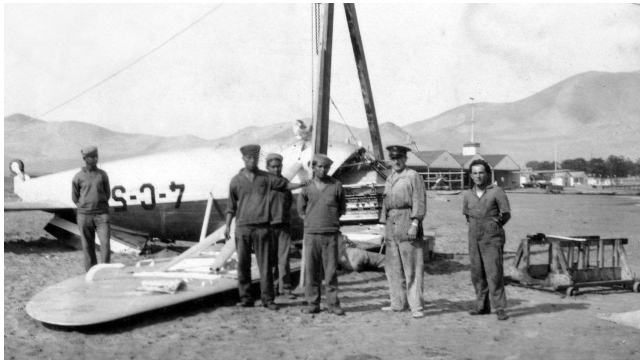
The narrow undercarriage was cause of more than one accident during the NiD-121 operational life with the CAP. This Nieuport, identified with serial 4-C-5 and assigned to the 4to Escuadrón Mixto, was damaged during landing at the beach of Alférez Carlos Huguet seaplane base in Ancón, in May 1935. (Photo: Author's collection)
