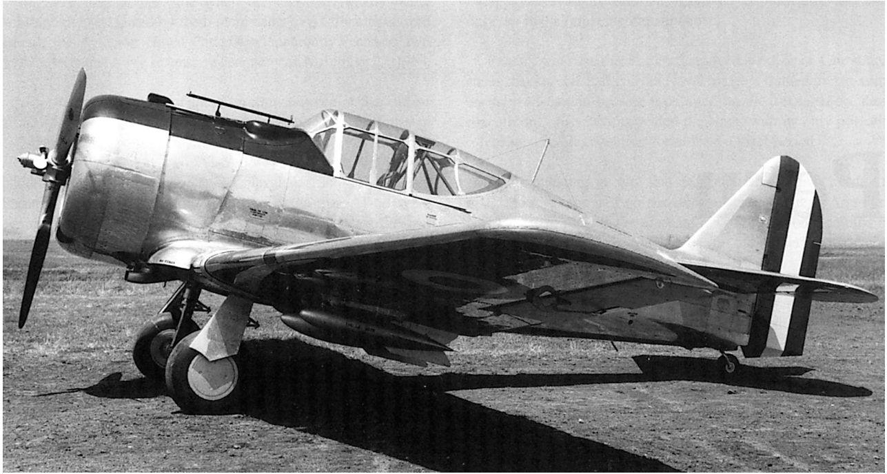
One of the Peruvian NA-50s, photographed at the North American Aviation plant, equipped with nose-mounted .30 Cal. machine-guns and carrying four bombs under each wing. (Photo: NAA via Dan Hagedorn.)
