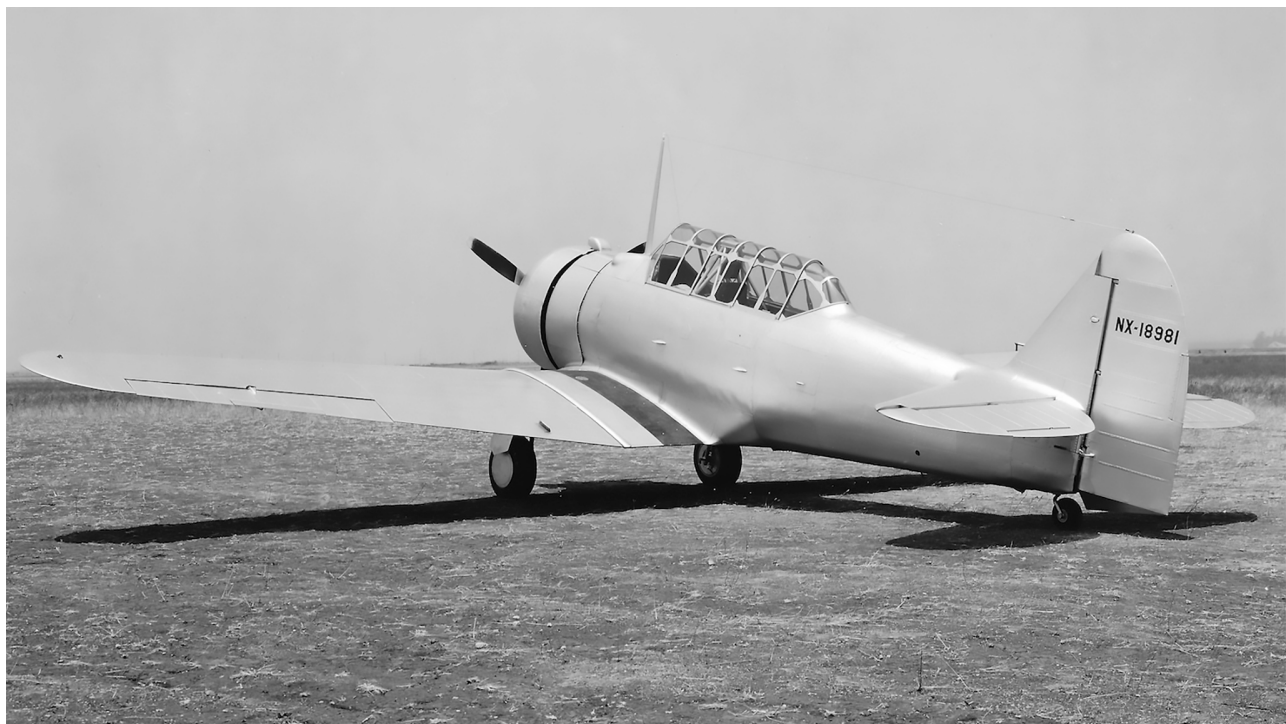
The NA-44 demonstrator, still equipped with a two-blade propeller. Later on, it was replaced by the characteristic three-blade prop. (Photo: NAA via Dan Hagedorn.)
