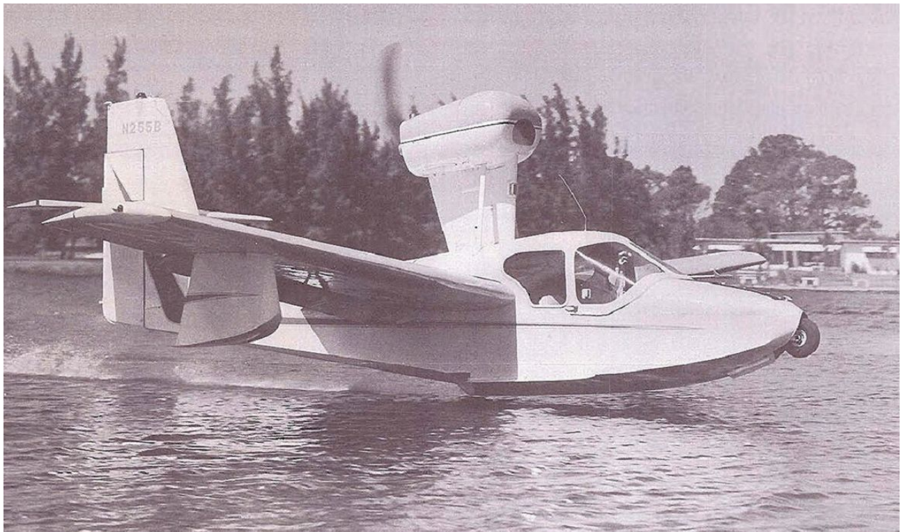
Another image of a Colonial C-2 Skimmer from the same sales brochure. Note that when retracted, the nose landing gear tire acted as a nose bumper. (Photo: A.A.S. Collection.)
