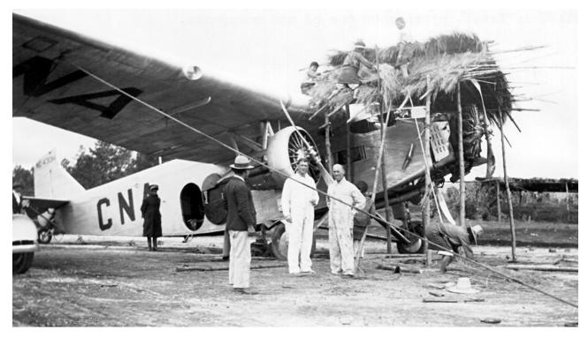
CNA's Ford 5-AT-C, U.S. registration N430H, undergoing repairs at the Sololá airfield after sustaining damage during a failed takeoff, in September 1935. (Photo: John Underwood via Gary Kuhn.)
