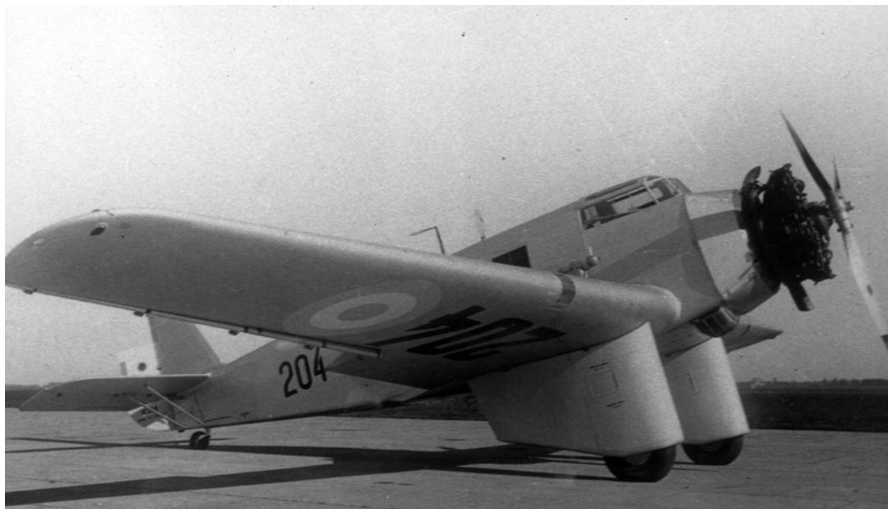
Ae.M.B.2 serial O-204 photographed shortly after the removal of her dorsal turret. The air-ram generator for the Telefunken radio can be seen above the wing. (Photo: Author's collection.)
