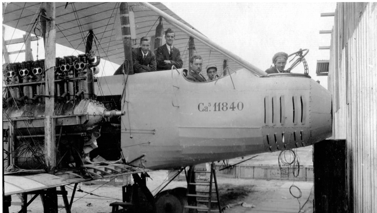
Unidentified civilians seen aboard this Caproni Ca.5 bomber at Maranga in May of 1921. Details of one of the three 200 hp Fiat A.12 6-cylinder water-cooled in-line piston engines fitted to this bomber can be seen in advantage. (Photo: Sergio de la Puente)
